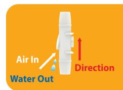
Siphon break must be higher than the water level in the reservoir.
