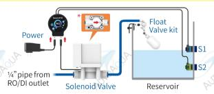
\*Water flow direction on the solenoid valve must be the same as the water flow direction.
