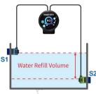
Step 2: Mount the green sensor (S2) and adjust the top sensor to the desired water level to refill\*.
